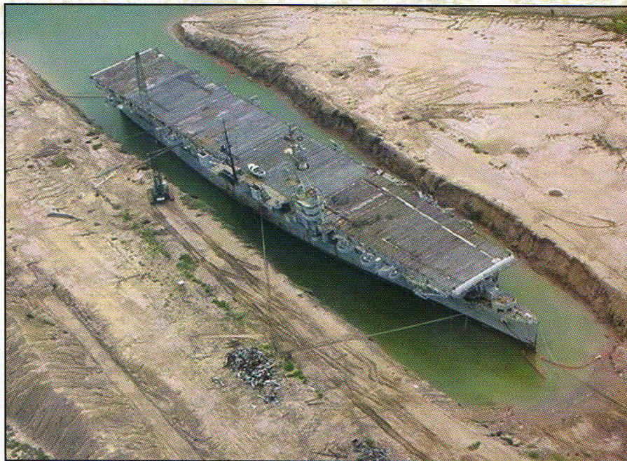
The ex-USS Cabot (CVL-28)/Spanish SNS Dedalo in a slip about to be stripped of readily available parts on deck and on the superstructure. As the ship is cannibalized further, a winch will pull it further into the slip and out of the water.
