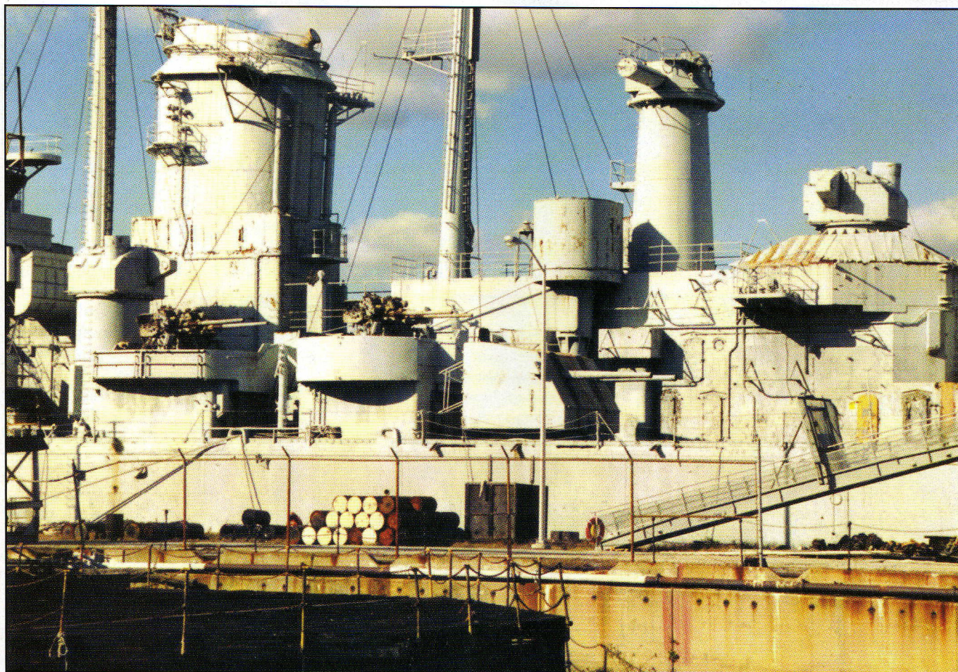
The Des Moines in Philadelphia, November 1999. Many items, valves and other pieces of equipment have been taken off the ship, and the 3-in/50-cal guns have literally been stripped. This is one of the liabilities of a ship in a reserve basin.
